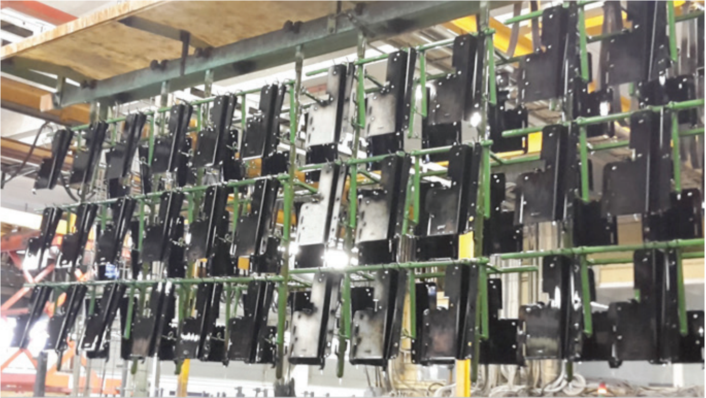
Fig. 20: Inhomogeneous formation of the passivation layer due to an indifferent solution movement
