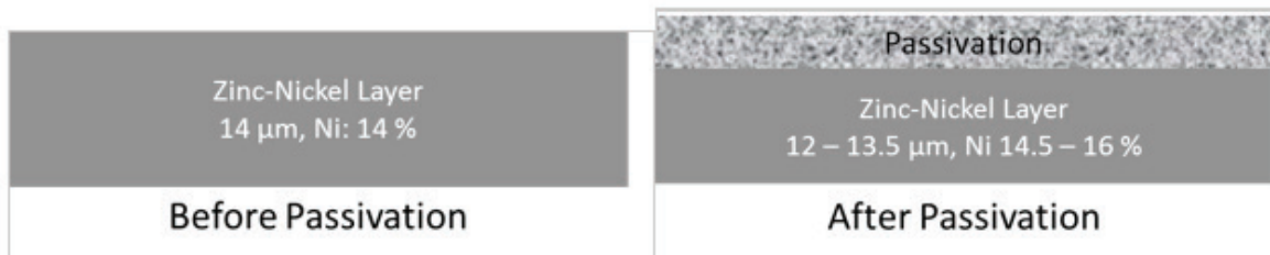
Fig. 9: Increase of nickel concentration in the layer and decrease of layer thickness during passivation
