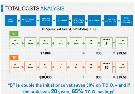
Figure 1 - Theoretical cost analysis for liners where "A" represents a commodity tank such as PP and "B" represents PVDF.
