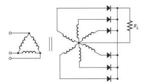
Drawing above shows a typical Delta primary main rectifier transformer with a six-phase star secondary. The output of the diodes in this case are positive and the center of the star is negative. Drawing courtesy of Google Images
