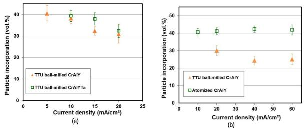
Figure 3 - Particle incorporation in the coating as a function of plating current density: (a) in the low current density range with ball-milled CrAlY and CrAlYTa powders, and (b) in the high current density range with ball-milled and atomized CrAlY powders.
