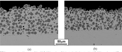
Figure 2 - SEM cross-sectional images of the Ni-CrAlY coatings fabricated with the atomized CrAlY powders at different current densities: (a) 10 mA/cm<sup>2</sup>; (b) 60 mA/cm<sup>2</sup>.
