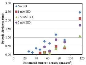
Figure 5 - Ni-W deposit thickness with varying amounts of BD.
