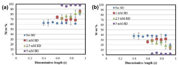
Figure 3 - Alloy composition as a function of cathode length: (a) nickel and (b) tungsten.
