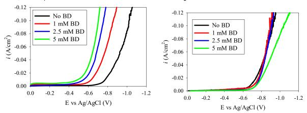
Figure 1 - Effect of BD on the polarization behavior of the (a) Ni-W electrolyte and (b) the Ni electrolyte.
