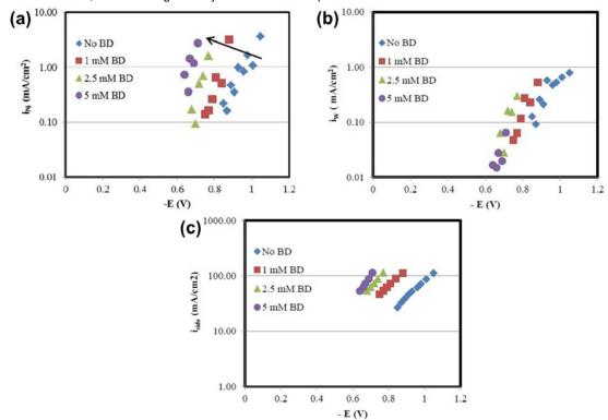
Figure 6 - Effect of BD concentration on (a) nickel, (b) tungsten and (c) side reaction partial current densities.
