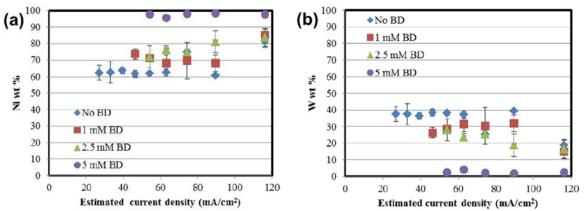
Figure 4 - Alloy composition as a function of current density: (a) nickel and (b) tungsten.
