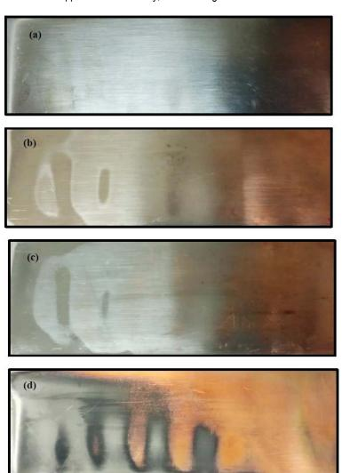
Figure 2 - Photographs of Ni-W deposit with varying amounts of BD at an average current density of -50 mA/cm<sup>2</sup>: (a) No BD, (b) 1 mM BD, (c) 2.5 mM BD and (d) 5 mM BD.
