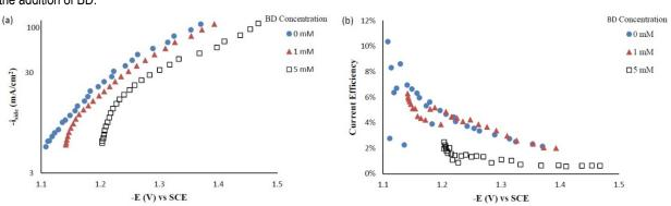
Figure 4 - Side reaction (a) and current efficiency (b) of Ni-W-TiO<sub>2</sub> composite deposition with variable BD concentration.
