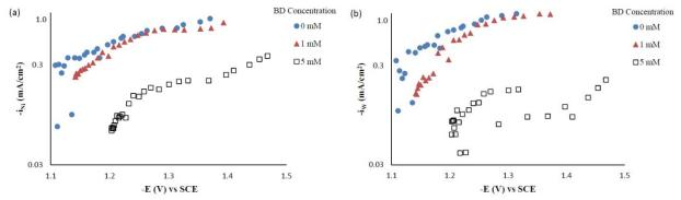
Figure 3 - Partial current densities of Ni-W-TiO<sub>2</sub> composite deposition with variable BD concentration: (a) nickel and (b) tungsten.
