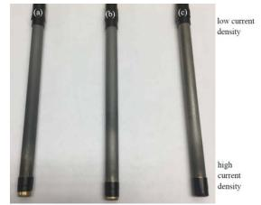
Figure 5 - Photographs of Ni-W-TiO<sub>2</sub> composite coatings plated with (a) 0 mM, (b) 1 mM and (c) 5 mM BD in the electrolyte for 30 min.
