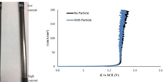
Figure 9 - Polarization curves of Ni-Mo deposition with and without TiO<sub>2</sub> particles.
