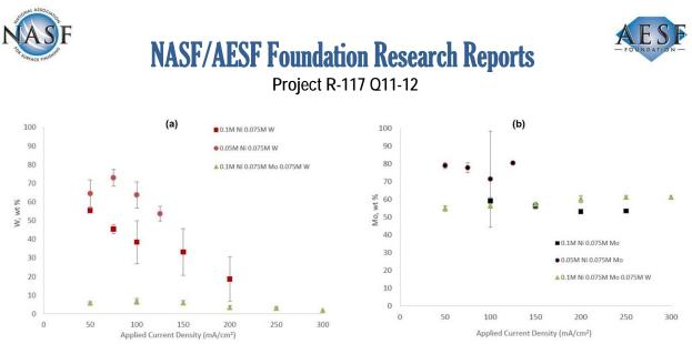
Figure 2 - (a) Tungsten composition in Ni-W and Ni-Mo-W deposits, and (b) molybdenum composition in Ni-Mo and Ni-Mo-W deposits produced at different applied current densities.
