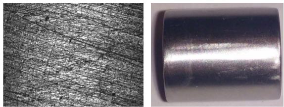
Figure 6 -Optical image and photograph of 0.1M Ni - 0.075M W deposit using an applied current density of 50 mA/cm<sup>2</sup>.
