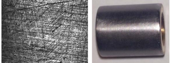
Figure 7 - Optical image and photograph of 0.1M Ni - 0.075M Mo deposit using an applied current density of 200 mA/cm<sup>2</sup>.
