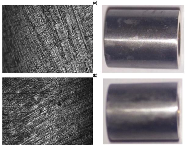
Figure 8 - Optical image and photograph of 0.1M Ni-0.075M Mo-0.075M W deposit using an applied current density of (a) 100 mA/cm<sup>2</sup> and (b) 250 mA/cm<sup>2</sup>.
