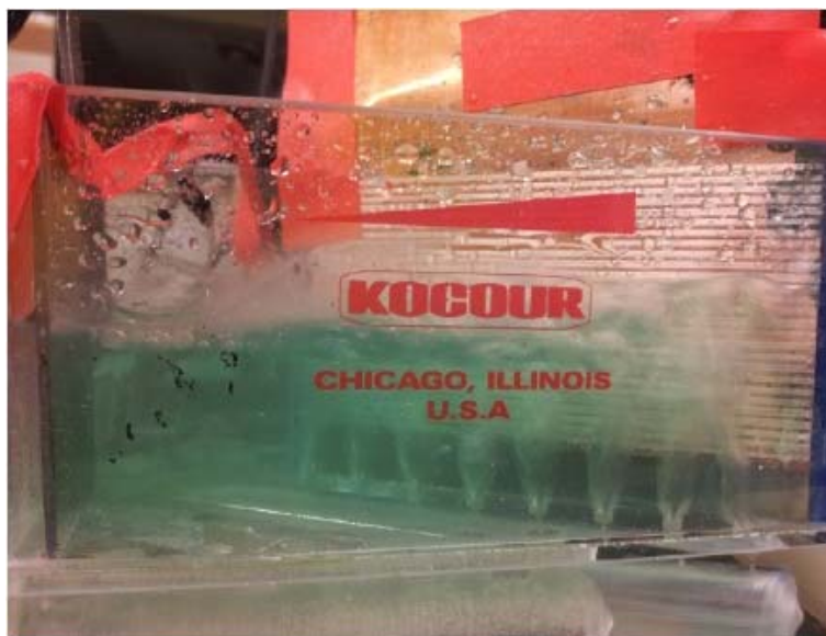
Figure 6 - Conventional Hull cell with air flow agitation.
