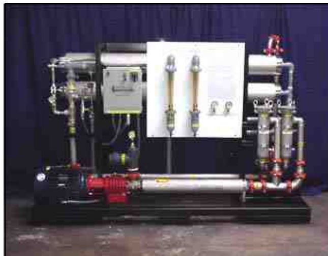
Figure 3. Perfection Plating's RO System
