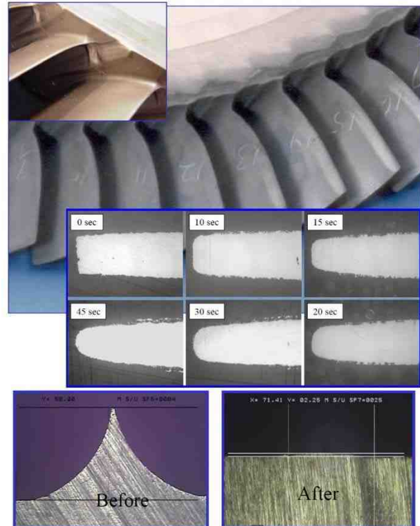
Figure 14 - P/PR electrolysis applied to aerospace components.
