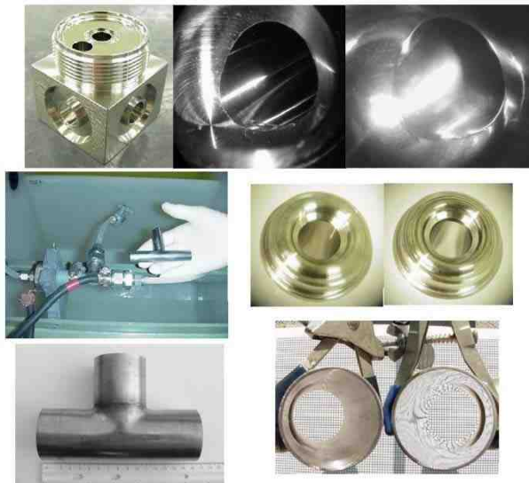
Figure 15 - P/PR electropolishing of stainless steel components.
