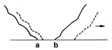
Figure 4 - Schematic representation of junction growth. Normal load deforms asperity so that contact occurs along line ab. When a tangential stress is imposed in the direction of the arrow, the junction grows, as shown by the dashed lines, and the two surfaces move together slightly.
