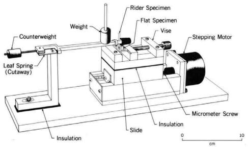
Figure 8 - Fretting test apparatus.
