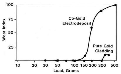
Figure 7 - Electrographic wear indexes from two-body, abrasive-wear runs with two 2-µm-thick gold coatings, namely, a cobaltgold electrodeposit on a 2.5-µm-thick nickel underplate on a copper-beryllium substrate and a pure gold clad inlay with a nickel interliner on a copper-nickel-tin alloy substrate (single-pass runs at various loads with a conical diamond rider).
