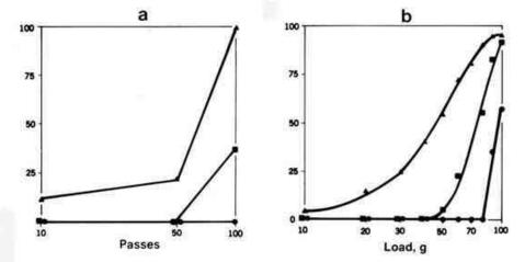
Figure 3 - Runs to determine the effect of surface roughness on wear for a 0.6-µm-thick cobalt-gold electrodeposit on a 1.5-µm-thick nickel underplate on copper flats abraded before plating to 3 levels of roughness (▲ 7.5 µm c.l.a.; ■ 0.38 µm c.l.a.; ● 0.1 µm c.l.a.). (a) adhesive wear with solid gold riders (100-g load); (b) two-body abrasive wear runs with a conical diamond rider (single pass).
