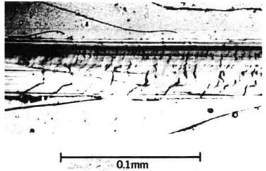
Figure 6 - Wear track on a 65/35 Sn-Ni electrodeposit 12 µm thick with a 0.43-µm-thick overplate of cobalt-gold alloy (diamond rider, 90° conical tip with a radius of 0.1 mm, single pass at a load of 200 g). Deposit shows brittle fracture.
