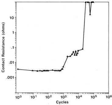
Figure 11 - Contact resistance vs. number of fretting cycles for a palladium rider (3.2 mm in diameter) tested against a palladium flat using a 20-µm wipe, a 50-g load, and a frequency of 4 Hz. The increase in contact resistance is due to the formation of frictional polymers.
