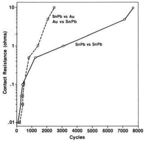
Figure 9 - Contact resistance vs. numbers of fretting cycles for tin-lead solder against itself compared to gold vs. tin-lead-plated contacts. The contacts were not lubricated (Wipe distance, 10 µm; normal load, 50 g).
