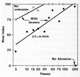
Figure 2 - Three-body abrasive wear runs with a 3.3-µm-thick cobalt-gold electrodeposit on copper with and without a nickel underplate (lubricated; 50-g load; coarse silicon carbide particles sprinkled on the flat).
