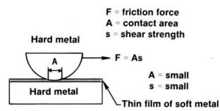
Figure 5 - The friction between metal surfaces can be lowered by depositing a thin film of a soft metal on a hard metal substrate (after Ref. 5). A coating of a metal that resists junction growth, such as electrodeposited cobalt-gold, will function in the same way as a soft metal film.
