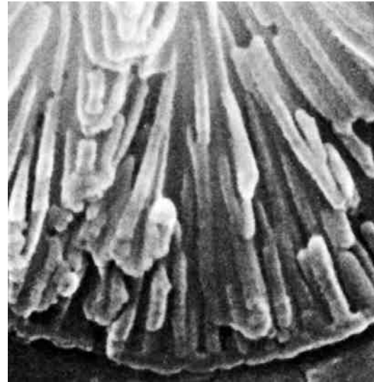
Figure 4 - Higher-magnification view of Fig. 3 shows pore branching and inclination of divergent pores.
