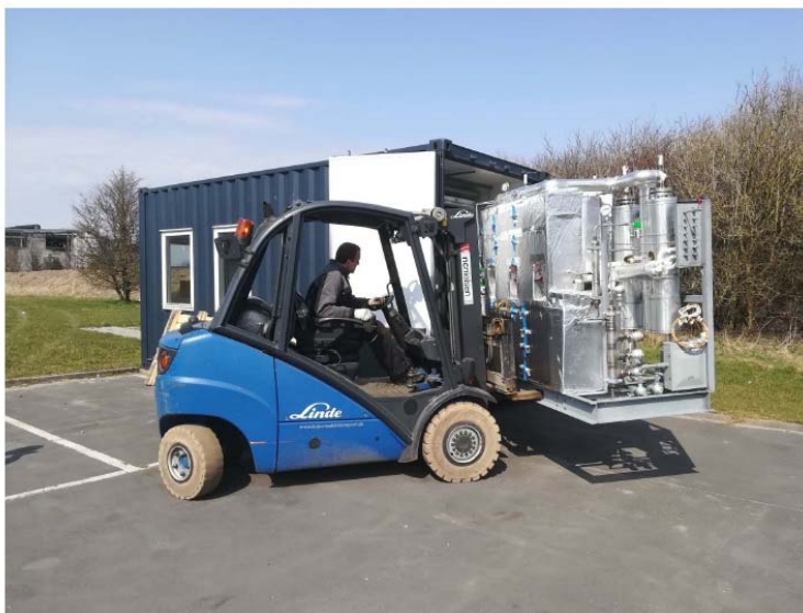
Slide 46 - Upgrading CO 2 to methane - Commercial reactor.
