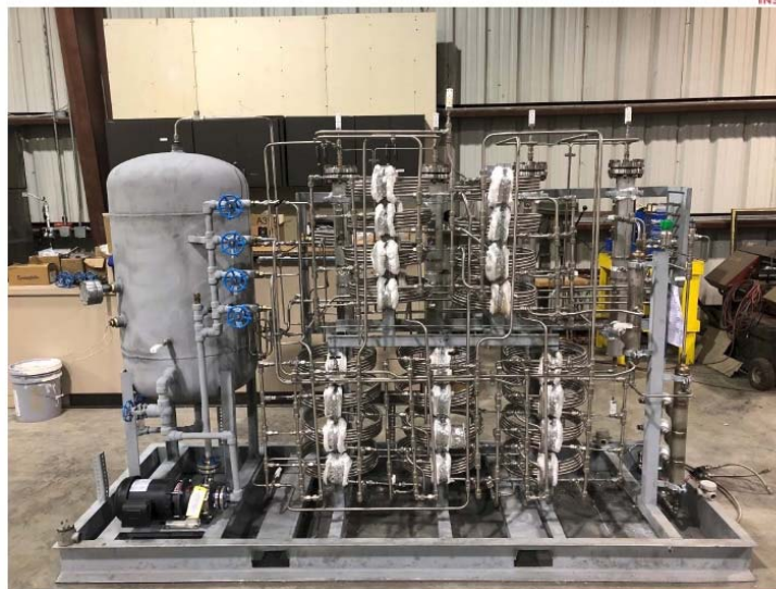
Slide 45 - Upgrading CO 2 to methane - Pilot reactor.
